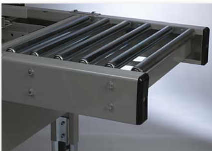
Infeed/Exit Conveyor – Ball bearing steel rollers in steel frame bolts to the 3M-Matic™ Case Sealer to provide a smooth transition in existing conveyor lines. Provides pack area surface at infeed. Available also in stainless steel.
