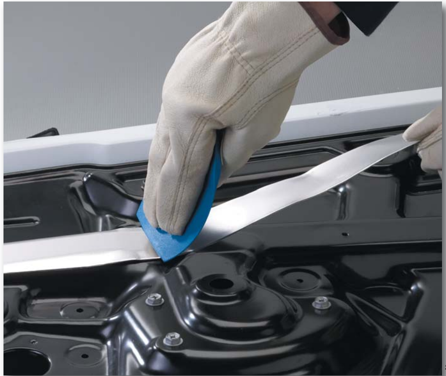
Applied with a 3M™ PA-1 Wiper to the inside of a car door, 3M™ Damping Foil 2552 effectively damps noise and vibration with as little as 10% surface coverage. Optimized acrylic on a dead soft aluminum constraining layer converts vibrational energy to negligible heat that readily dissipates.
