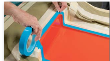
For composite masking, 3M fine line (see page 8) overtapes 3M crepe masking tape for gelcoat color separation.
