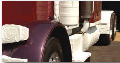
During production and transit, white polypropylene tape protects truck surfaces such as rocker panels, chrome finishes, mirrors, lights and lenses.
