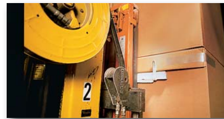
With glass yarn reinforcement, high tensile strength, and low stretch, Scotch® High Strength Filament Tape 890 is designed to hold the lift flap in place on Basiloid containers.
