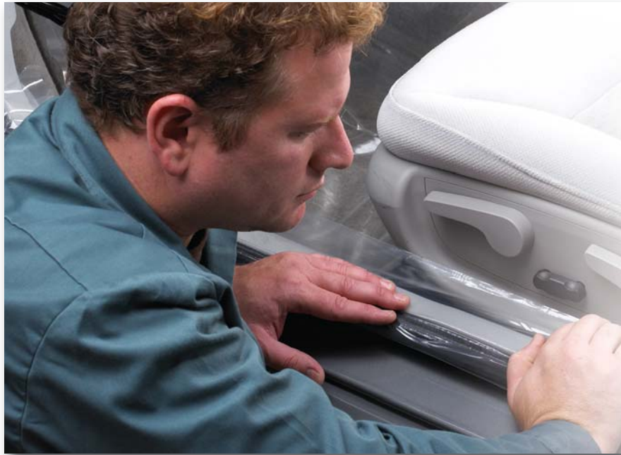
During manufacturing and transport, transparent 3M™ Polyethylene Protective Tapes protect many finished automotive interior surfaces from abrasion, nicks, and scratches. Clear acrylic adhesive holds with very low tack for easy removal.
