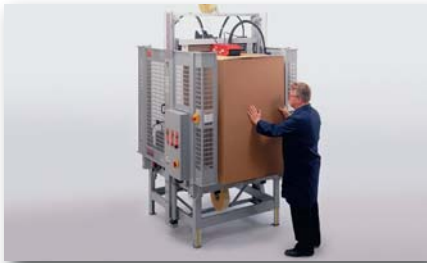
800rks – King-size automatically adjusts for case sizes up to 30" wide by 48" high. Upper and lower side belt drives ensure taping accuracy up to 12 cases/minute. 48 mm to 72 mm tape widths.
